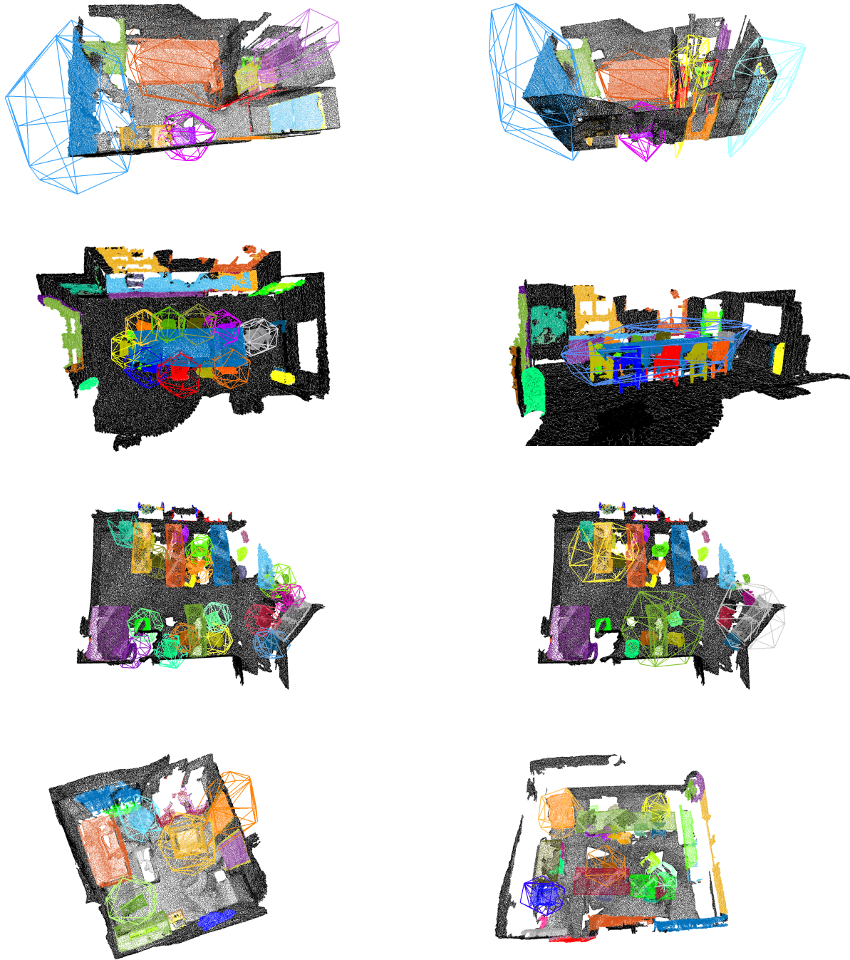
Figure 11. Visualization of convex hulls on ScanNet – Note we visualize only some of the hulls to reduce visual density. We visualize the wireframe of the hulls for better visibility. And we color the points according to the instance prediction.
