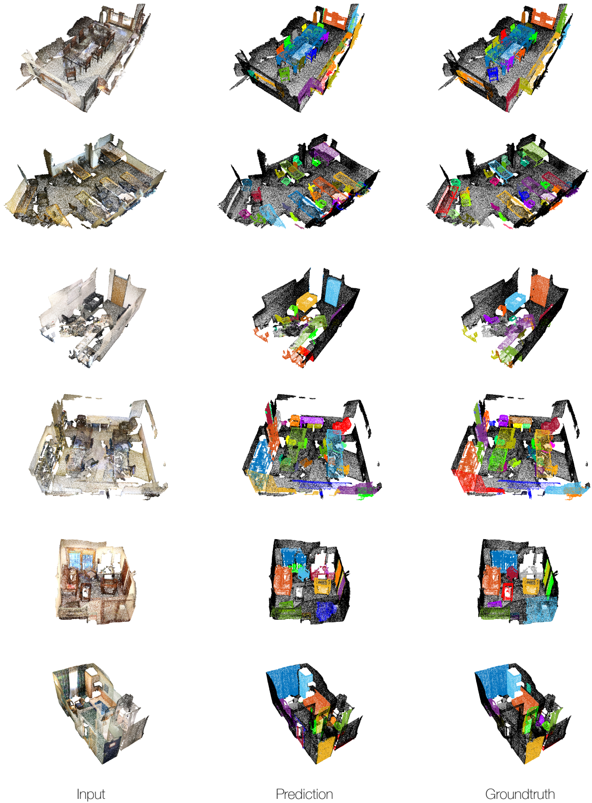
Figure 12. More qualitative results on ScanNet – Instance segmentation results in the validation set.
